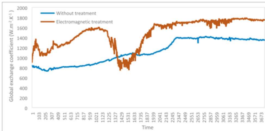
Fig. 19. Variation of the global exchange coefficient in the absence and presence of Electromagnetic resonance field of low intensity and low frequency.
